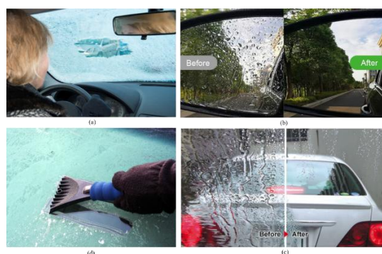
Figure 2: (a) Frost formation is one of the main challenges of cold region drivers. Effect of superhydrophobic coating on (b) rear-view mirror and (c) front windshield. (d) Mechanical defrosting is only suitable for when the car is in park mode.
